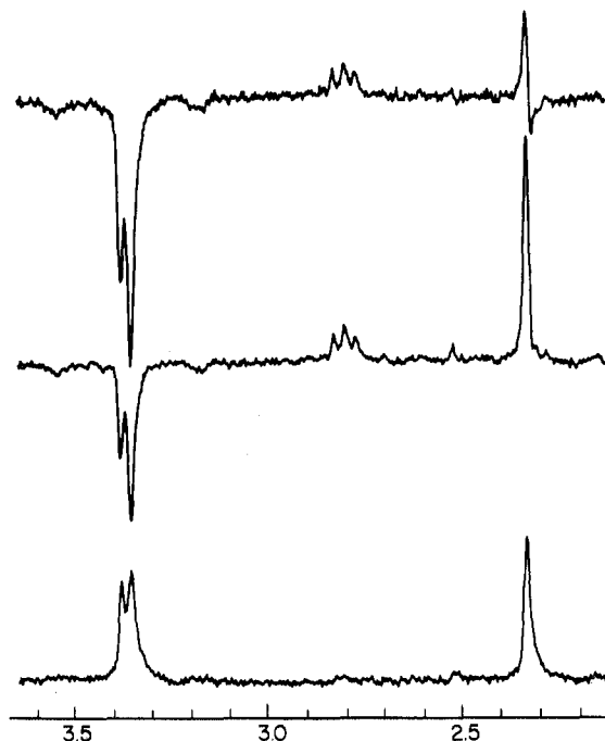
Figure 1. ^1\text{H} NMR spectrum (90 MHz) of p -methylbenzyl benzyl ketone in the dark (bottom) and during UV irradiation (center). The top trace represents the difference between the dark spectrum and that observed during irradiation.
